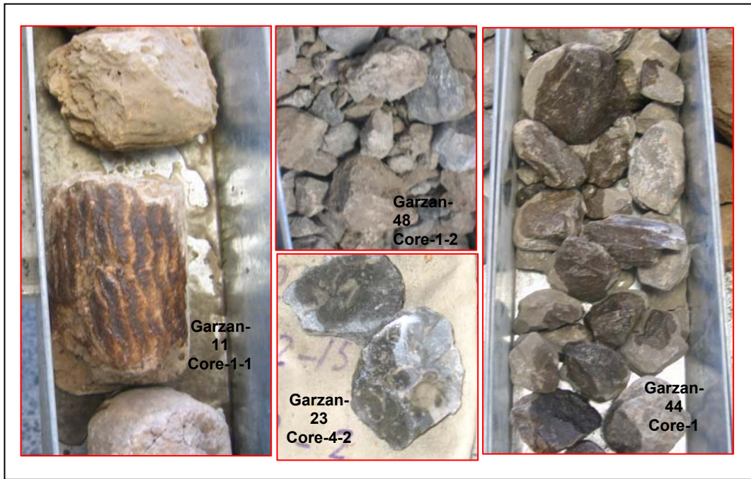
Figure 7: Photographs of the condition of the cores of Garzan Germik oil field wells.
